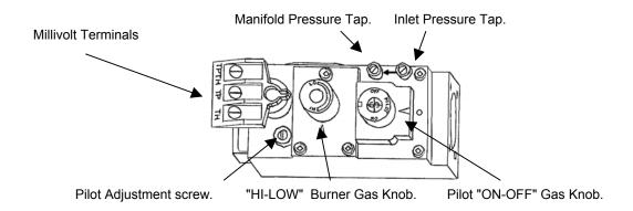
The appliance and its shutoff valves must be disconnected from the gas supply piping system during any pressure testing where the pressure exceeds 1/2 PSIG (3.45 kPa) or damage will occur to the valve.
